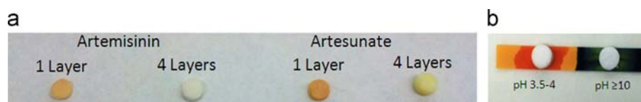
Fig. 3. (a) pH dependence of FRTR colorimetric test on paper. (b) pH test of 1 M NaOH solution added on two layered paper chips that were preloaded with citric acid buffer (left) and a blank (right).
