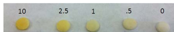
Fig. 4. Semi-quantitative data utilizing the designed paper test device. From left to right: decreasing concentrations of artesunate from 10 mg/mL to 0 mg/mL.
