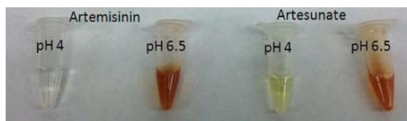
Fig. 2. pH dependence of FRTR colorimetric test in solution. Artemisinin turns an orange color at pH 6.5, while giving no color at a pH of 4. Artesunate turns an orange color at pH 6.5, while giving a yellow color at a pH of 4.
